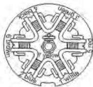
7-way trailer plug car end, rear view
