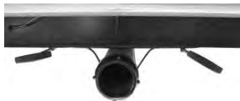
Black/Grey Tank Drain and Valves
